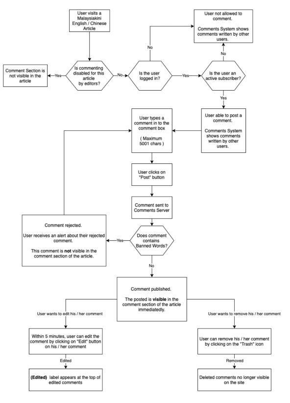
have been comprehensively explained by an expert in his report in Enclosure 58. The process of commenting can be summarized in the diagram below.<sup>23</sup>
